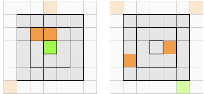
Figure 3. A core’s state depends on the states of neighbors in its inner and outer annulus spanning 3-by-3 and 5-by-5 16-pixel patches, respectively.
